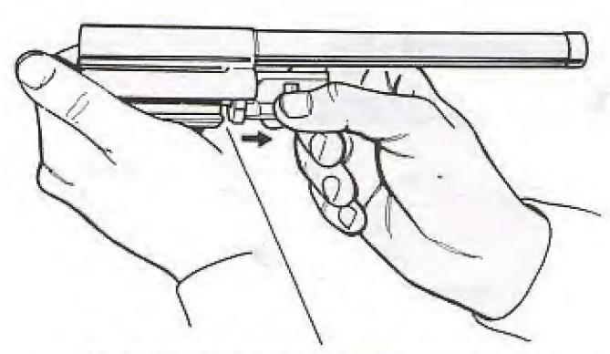
When bolt rollers are depressed bolt assembly should move forward ¼ "inch.
